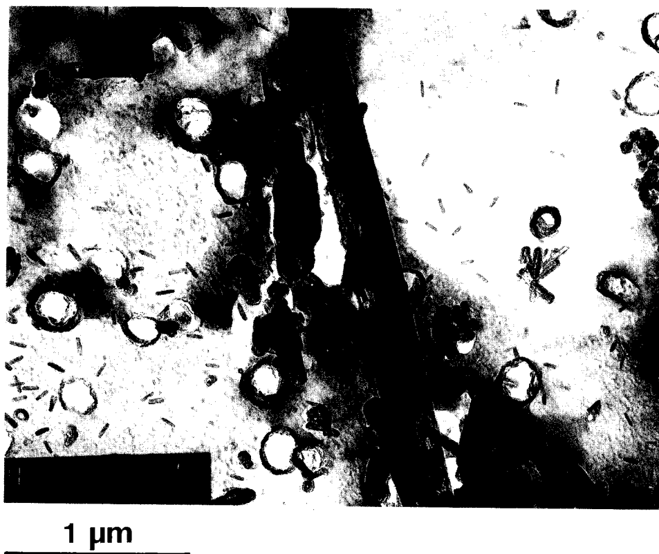
Figure 3. High magnification transmission electronmicrograph of one big fiber and several single crystal microfibers.
