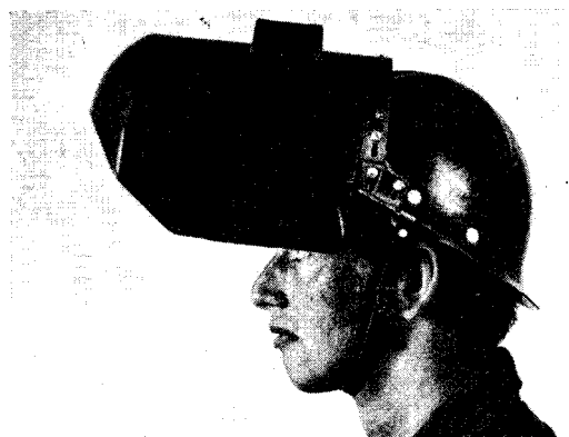
Fig. 1. Skullguard/welding helmet combination. The subject wore the device during the entire experimental procedure. (Photo A. Rosengren)
