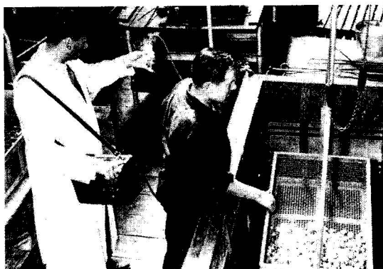
Figure 1. Air sampling with an impinger in the operator's zone and a hand-activated portable pump.
