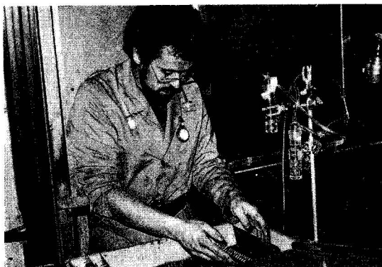
Figure 3. Operator equipped with a charcoal tube (inside a plastic holder), a badge, and a filter cassette. Beside him a sampling system with conventional impingers to collect ethanalamine.
